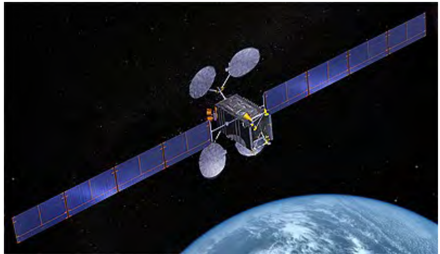
ABS-3A, launched last March, is currently in an extended orbit-raising phase to geostationary position at 3°W. It is equipped with 48 x 72 MHz C & Ku-band transponders and will offer expanded communications and broadcast capacity connecting the Americas, Europe, the Middle East, Africa, and the North Atlantic Ocean. (image: ABS)
