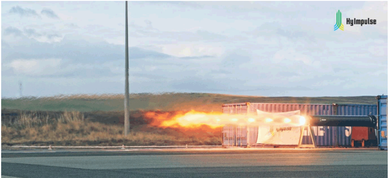
Firing of the SR75 motor during a qualification test of the HyImpulse test facility in the Shetland Islands.
