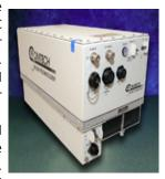
amplifier. We have full mil qualification. V-Band is an emerging frequency of interest due to the vast available bandwidth and the availability of V-band hardware. Comtech Xicom offers a 250W V-Band amplifier for gateway service.
