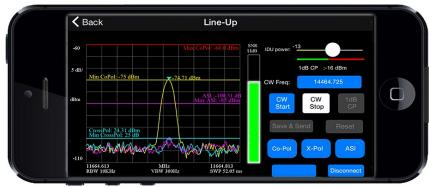
Integrasys Satmotion Pocket is a unique VSAT Auto Commissioning System for minimizing the deployment time, effort and interference intra-satellite such as CrossPol and inter-satellite such as Adjacent Satellite Interference (ASI).
