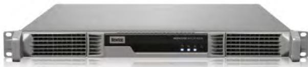
will be showcasing at Satellite and CABSAT its most advanced VSAT modem to date – the first on the market to support wideband DVB-S2X, the **Newtec MDM5000 Satellite Modem**. The MDM5000 is capable of receiving forward carriers of up to 140 MHz, and processing over 200 Mbps of throughput. On the return channel, it supports SCPC, TDMA and Newtec's unique Mx-DMA™, up to 75 Mbps.
