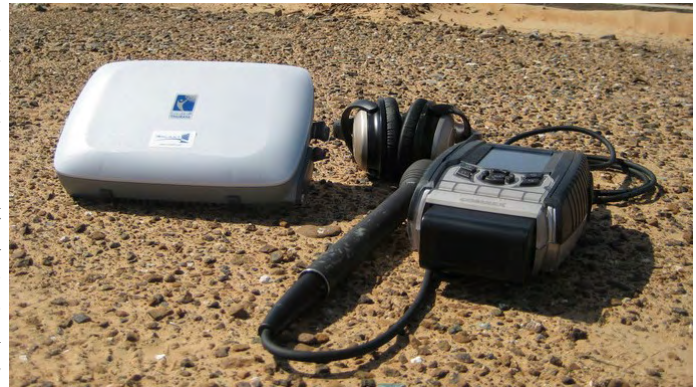
Equipment for Thuraya’s IP broadband Internet service. (photo courtesy of Thuraya).
