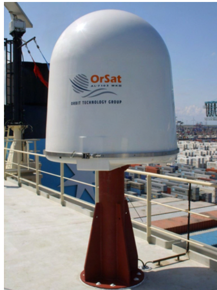
Orbit's OrSat stabilized antenna for maritime applications. (photo courtesy of Orbit)
