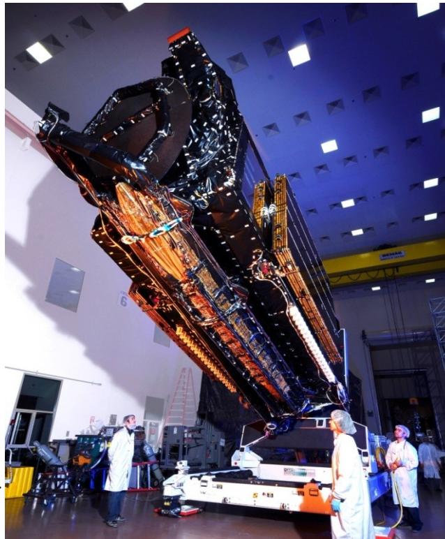
TerreStar-1 pictured here, has an 18-meter antenna reflector, is the largest commercial satellite ever launched to date. (photo: Space Systems/ Loral)
